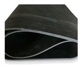
Noisestop Barrier shield is a versatile high density mass loaded vinyl barrier. Suitable for use in soundproofing walls, floors, ceilings and enclosures. Apply to plasterboard and other sheet materials to reduce vibration. The high density compound increases the mass of the area it is applied, reducing sound transfer through the structure. With properties similar to sheets of lead Barrier Shield is used in many areas that require noise reduction with minimal space loss.
