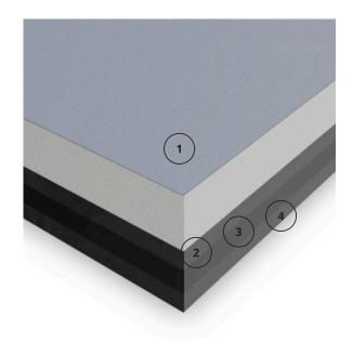
Noisestop Acoustic Panel comprises four layers that are pre-bonded for ease of installation. The board's surface is a 12.5mm acoustic plasterboard with a tapered edge, allowing for a plaster skim or taping and filling before decorating. The triple-layered acoustic membrane on the back of the panel is a 5kg mass-loaded vinyl, a 5mm closed-cell acoustic grade foam, and another 5kg mass-loaded barrier layer.
