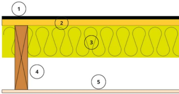
Mass-air-mass resonant frequency = -81 Hz
