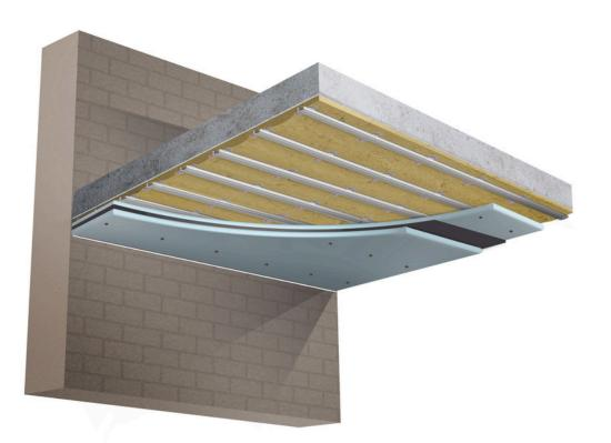
ACOUSTICLIP CONCRETE CEILING SOUNDPROOOFING SOLUTION
