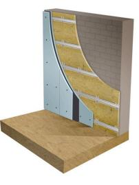
Mass air resonant frequency = 42Hz Panel size = 2.7m x 4.0m Partition surface area mass = 152kg/m2
