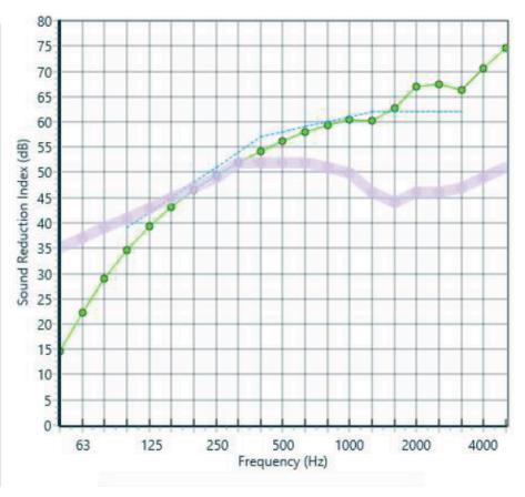
The higher the figure for airborne, the better the performance. The lower the figure for impact the better the performance.
