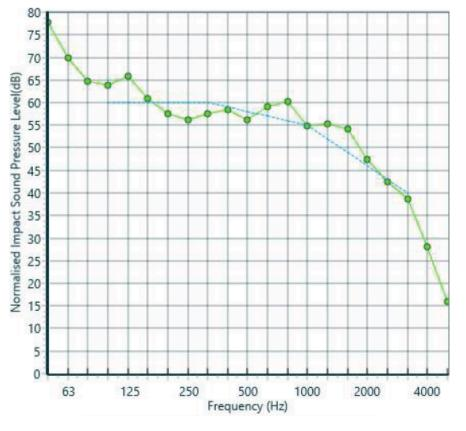
The higher the figure for airborne, the better the performance. The lower the figure for impact the better the performance.
