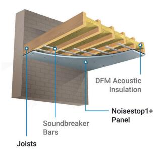
Mass-air-mass resonant frequency = = 81 HzPanel Size = 2.7 m x 4.0 mPartition surface mass =  $202 \text{ kg/m}^2$
